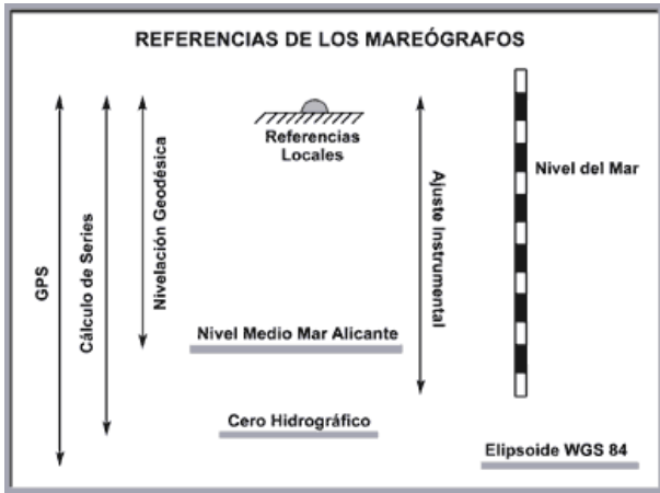
Figure 9. Relation between the different height references in a tide gauge.
