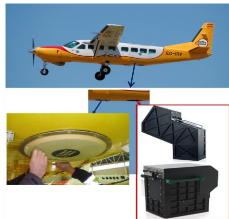
Figure 1. Thermal and VNIR hyperspectral sensors and radiometer installation onboard ICC airplane
