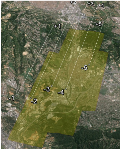
Figure 1 - TASI flight plan over Rubí
